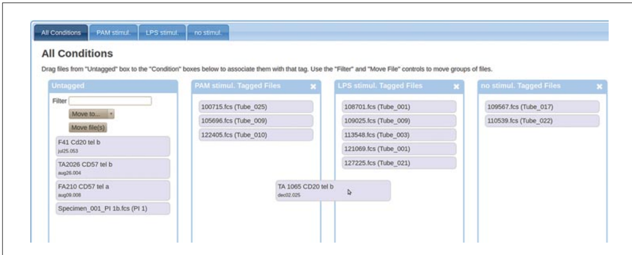
Figure 10.18.15 Conditions assignment. Experimental variables (e.g., sample stimulation conditions) can be assigned to FCS files by dragging and dropping the file labels to appropriate boxes.
