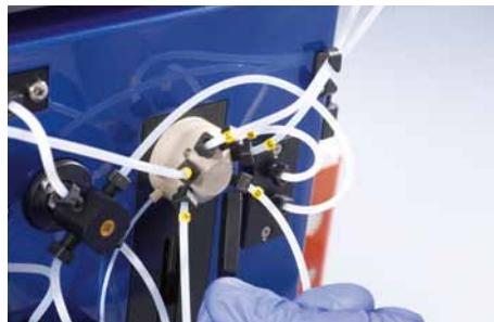
Figure 7.21: Unscrewing the tubing connected to the dilutor valve.
