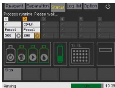
Figure 6.30: Monitoring the status during cell separation. Sample processing at position 1 is completed (white color). Sample at position 2 has finished the separation and is now performing a Rinse.
