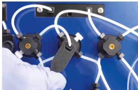
Figure 7.15: The valve cover-screw is unscrewed.
