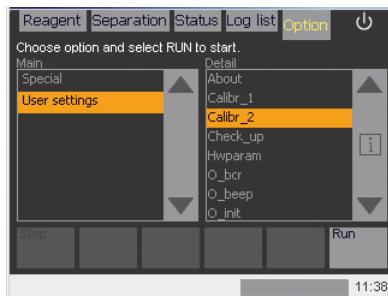
Figure 11.11: Performing Calibration 2 by selecting program "Calibr\_2".
