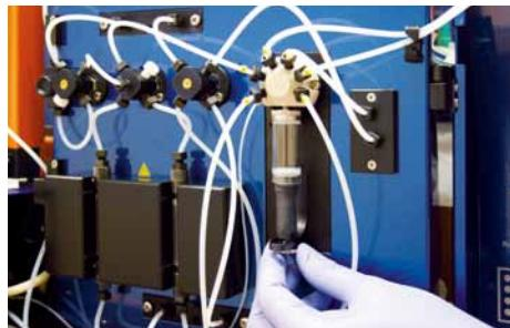
Figure 7.9: The plunger is placed in its fitting in the plunger holder. The plunger screw is fastened.
