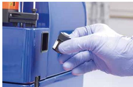
Figure 6.8: Scanning a reagent vial using the 2D code reader. In this example, the vial “CD4 MicroBeads, human” was scanned.
