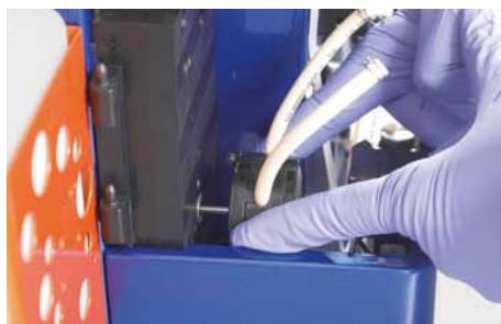
Figure 7.30: Detachment of the pump head.
