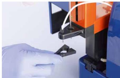
Figure 7.2: Removing the finger guard for cleaning.
