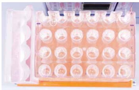
Figure 3.12: Positioning the Chill 5 Rack adjacent to a MACS Reagent Rack 4 on the MACS MiniSampler.
