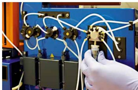
Figure 7.6: To remove the pump syringe the top screw must be turned counter-clockwise.
