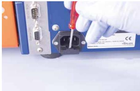
Figure 7.32: Removing the fuse holder.
