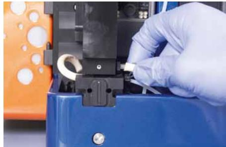
Figure 7.10: Remove the peristaltic pump tube from the washing station.
