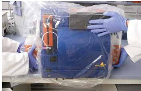
Figure 3.3: Positioning the autoMACS Pro Separator securely onto a laboratory bench.
