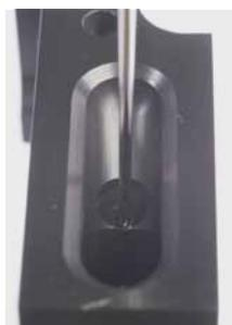
Figure 11.5: Test calibration of the needle arm position in the washing station. The position of the uptake needle should appear as shown above.
