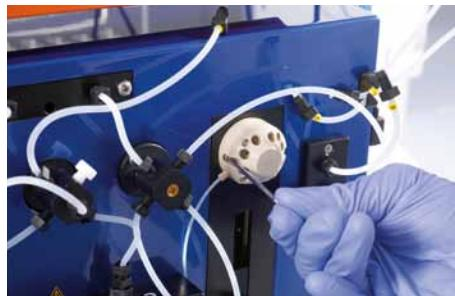
Figure 7.22: Unscrewing the dilutor valve's socket screws.
