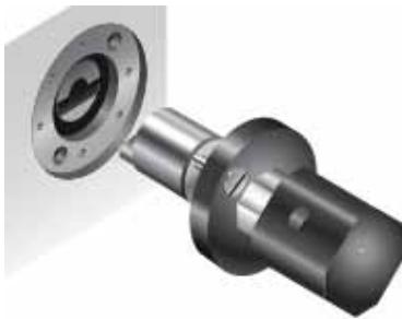
Figure 7.20: Inserting the new valve.
