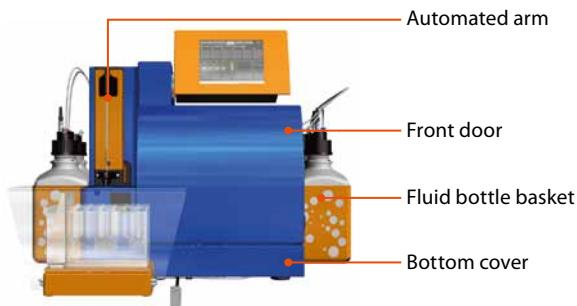
Figure 10.1: Front view of autoMACS Pro Separator.
