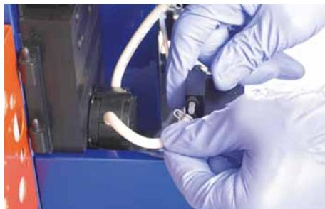
Figure 7.29: Disconnecting the tubing from the waste distributor.
