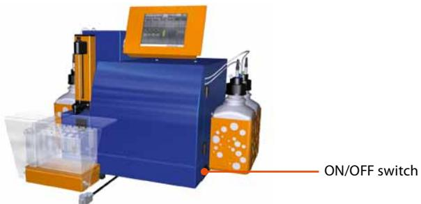
Figure 3.14: Location of the ON/OFF switch.
