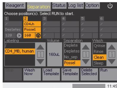
Figure 4.19: (Top) "Qrinse" program was selected. (Bottom) The "Clean" program has been enabled and was selected as the last wash program.
