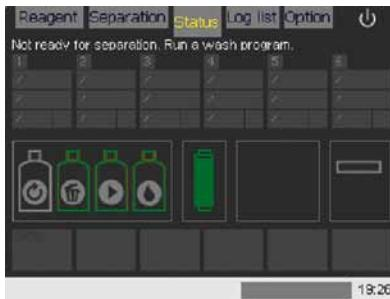
Figure 3.27: The “Status” menu. The fluid level status and column are green for ready. A wash or instrument prime has not yet been performed.
