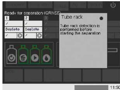
Figure 4.11: Tube rack status text box: No rack is detected until cell separation is performed.
