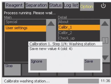
Figure 11.6: Saving new settings for calibration of the washing station.
