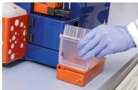
Figure 3.11: Securing the MACS Reagent Rack 4 onto the MACS MiniSampler.
