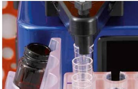
Figure 11.8: The uptake needle should be positioned as shown above.
