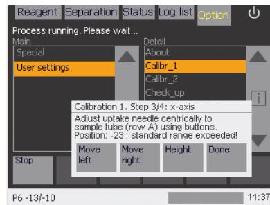
Figure 11.9: Adjust MiniSampler position.
