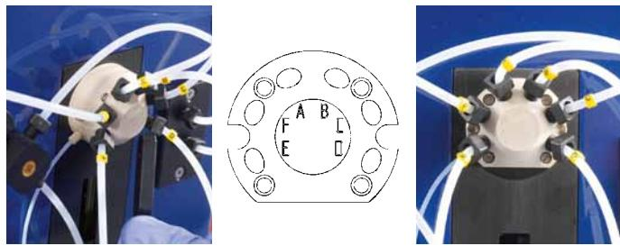
Figure 7.24: Connect tubing to the diluter value as shown above.
