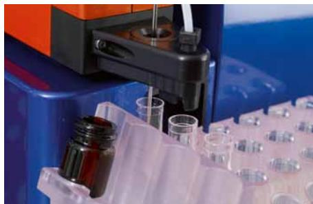
Figure 3.17: Test calibration of the needle arm position in the Chill Rack positions.
