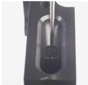
Figure 3.16: Test calibration of the needle arm position in the washing station.
