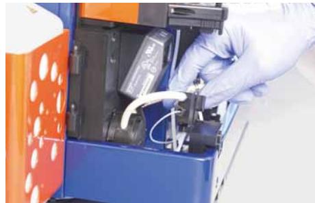
Figure 7.28: The draining tube is attached.
