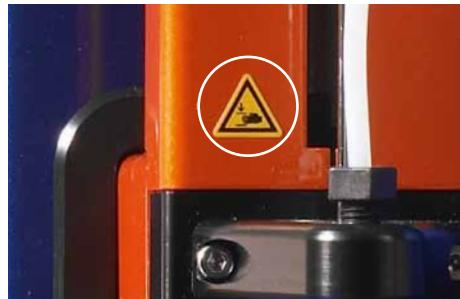
Figure 1.2: Open circle shows warning sign for hazard of crushing and shearing.
