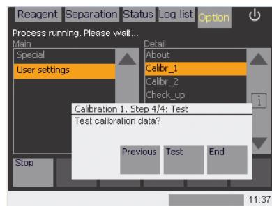
Figure 11.10: It is important to test the new calibration settings. To navigate back through the calibration steps, select "Previous".
