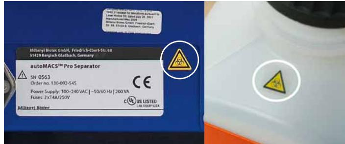
Figure 1.4: Warning signs for biohazard located on lower facing panel of the autoMACS Pro Separator (left) and on top of autoMACS Pro Separator fluid bottle (right).
