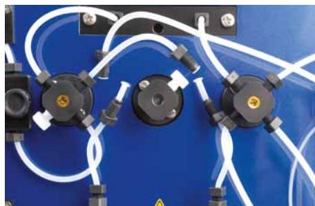
Figure 7.16: The valve cover-screw is unscrewed. Tubing and valve port locks or blind screws are detached.
