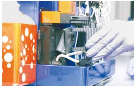
Figure 7.26: Disassembly of the washing station.
