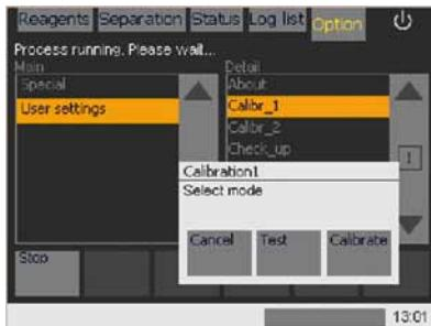
Figure 11.3: Performing calibration of the needle arm:
