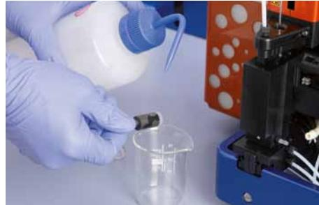
Figure 7.7: Washing the pump syringe with distilled water.
