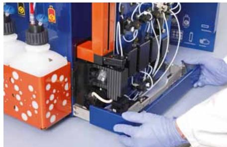
Figure 7.14: The bottom cover must be removed for access to the lower valve.
