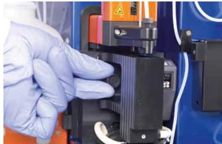
Figure 7.11: Unscrew the thumb screw.
