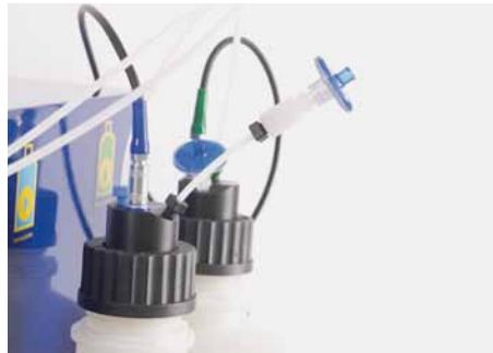
Figure 7.31: Hydophobic air filter attached to a fluid bottle.
