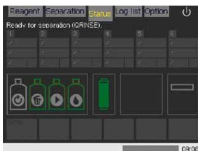
Figure 3.30: Status of the fluid bottles is green for ready.
