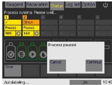
Figure 6.31: Select “Stop” to pause cell separation. To continue cell separation select “Continue”. To cancel the entire procedure, select “Cancel”.
