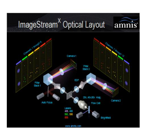
(Left) Examples of applications enabled by this powerful technology. (Right) How it works: ImageStream<sup>X</sup> Layout: The fluidics work in a similar way to all flow cytometers with a sheath stream to focus the cells before they pass through the lasers. The fluorescence and brightfield images are separated on to the detector camera. In order to create a higher image contrast the cells are tracked pixel by pixel down the detector surface and reconstructed by the software (Inspire).
