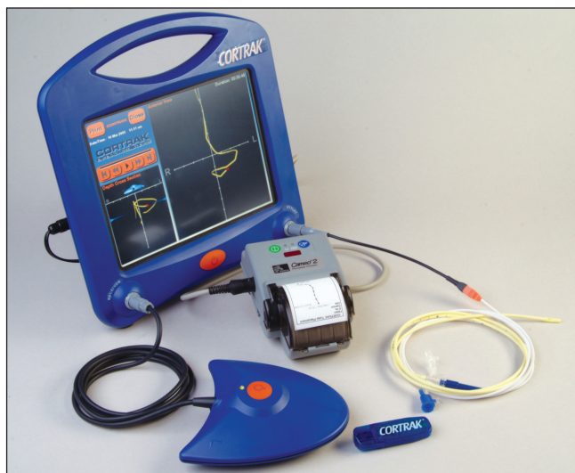
Figure 2. Cortrak Enteral Access System. ( www.corpakmedsystems.com/product_main/cortrak.html )
