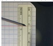
Figure 4. Applying a Kirschner bow to the end of a smooth pin inserted in the distal femur. The ruler is placed below the pin. The Kirschner bow is used to apply weight to the end of the pin. Deflection is measured to the nearest 1/10th millimeter.
