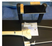
Figure 2 shows the traction model used for testing photos of the pin and underlying ruler/graph paper at each 5 lb increment in weight.
